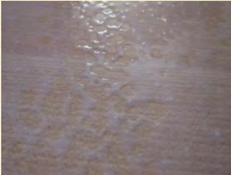
Laminated wood bedside table coated with NanoCote HD-WR (before curing).
