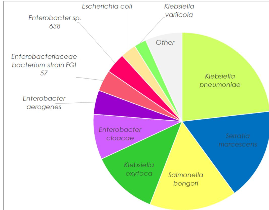
Example of biofilm composition from the small-scale drain model
