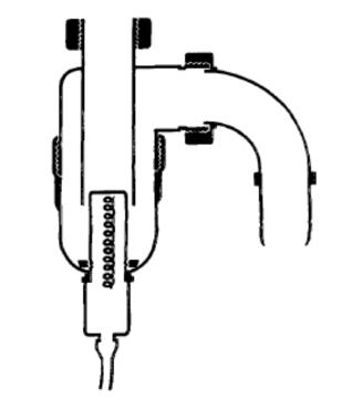
Fig. 2-Diagram of waste-trap unit with cylindrical electric heating element.
