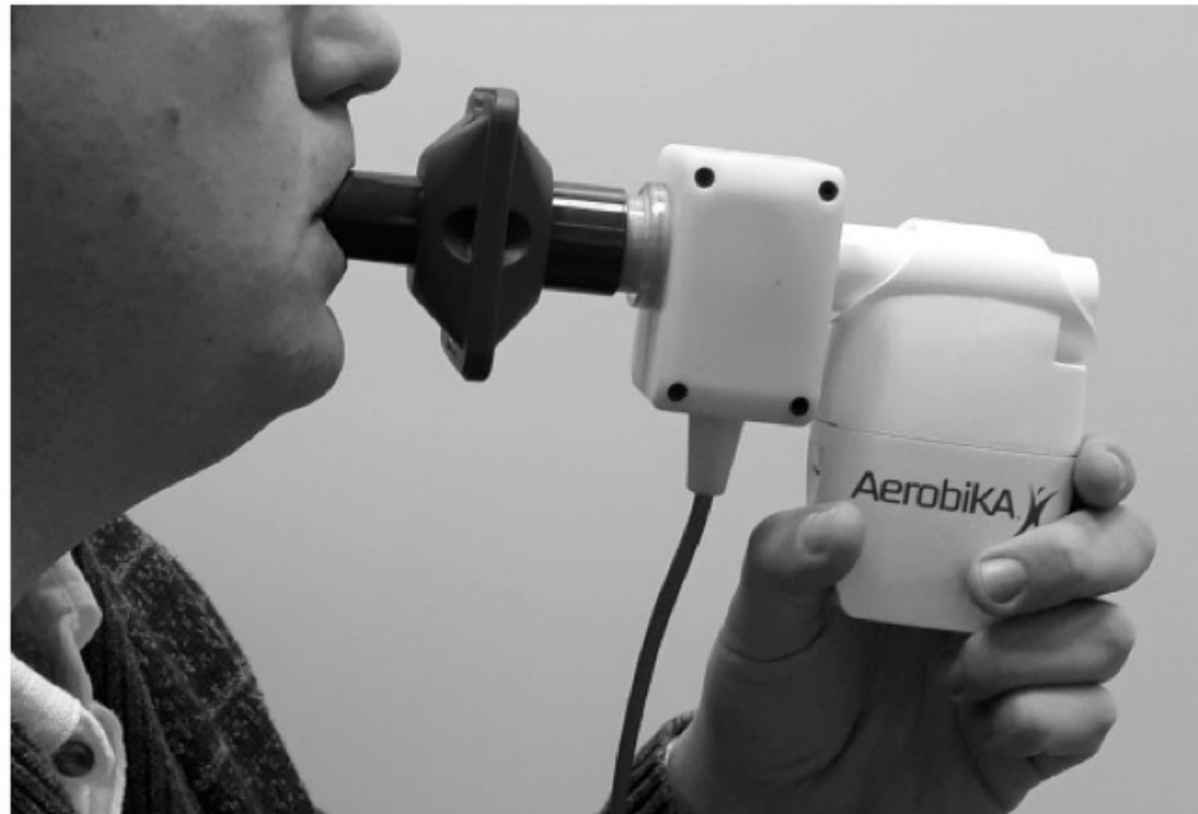
Figure 20: Author (KJOS) demonstrating the flow and pressure sensor positioned in-line with the OPEP device with anti-viral filter
