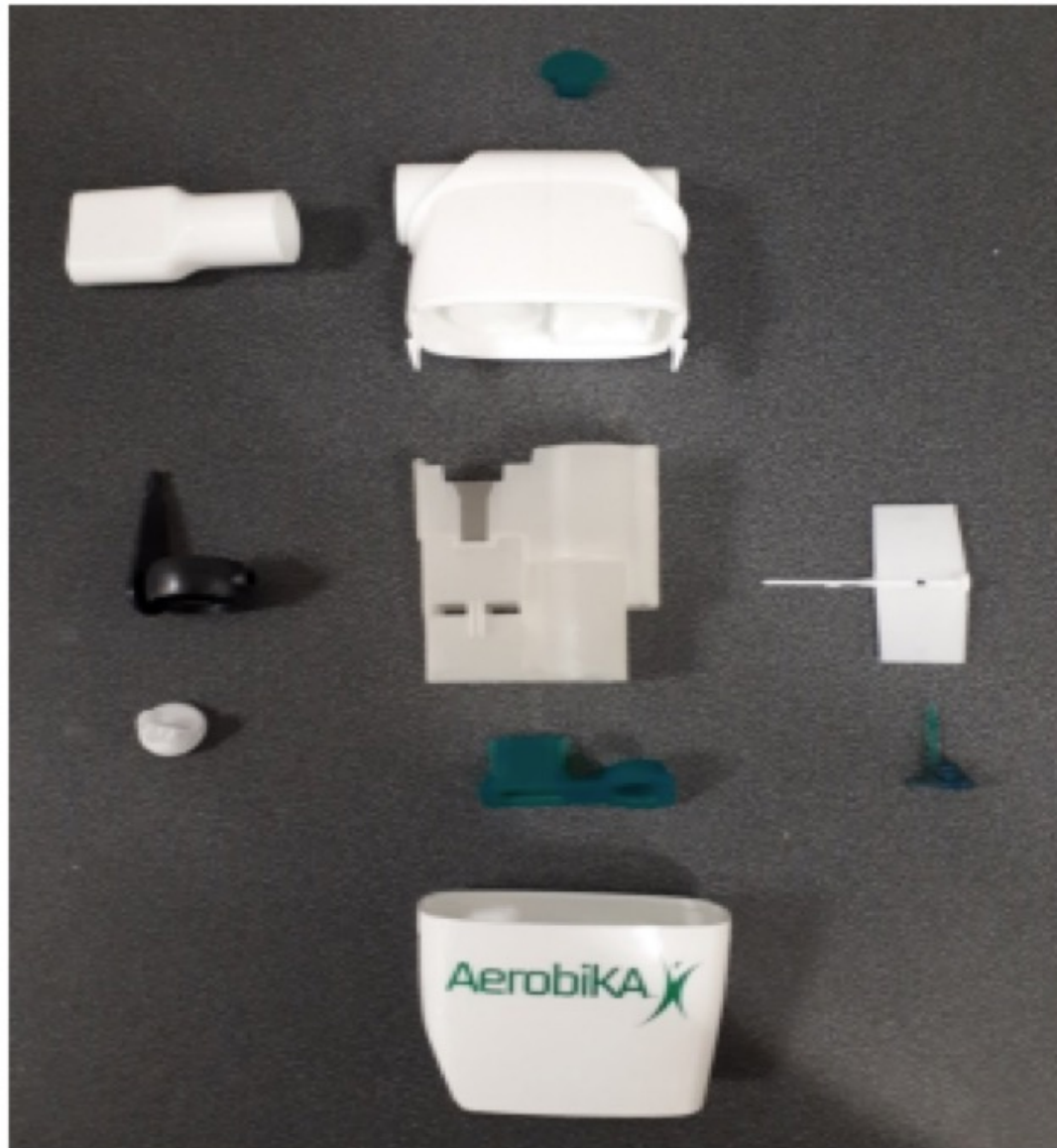
Figure 13: An Aerobika® device disassembled into all 10 individual components
